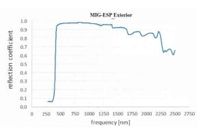
Spectrum of the diffuse refelctance of the sample ,ESP Außen'.
